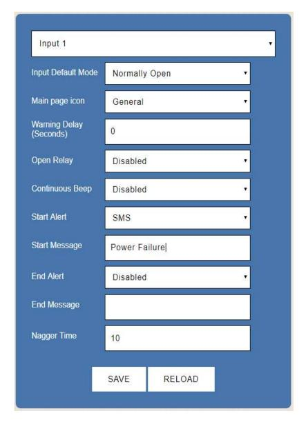
In the upper field you should choose the input number. In controllers that have a Power Supply/Charger that alert using a dry contact in any case of power failure, the first input will use for indication on power failure.
