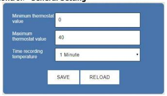
The minimal and maximal values of the thermostat is only for display in the main page of the controller.
