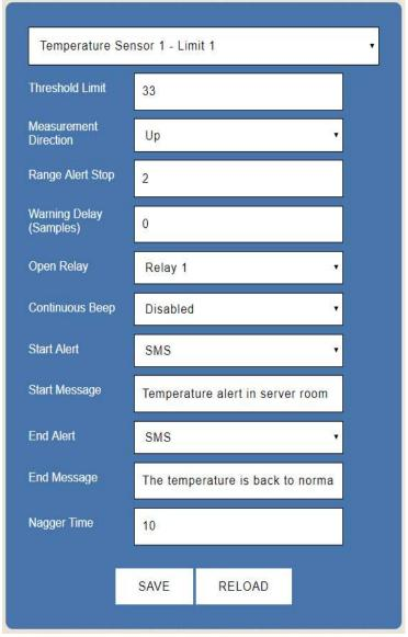
In the upper field you should choose the name of the sensor. Note that for each sensor you can define 2 temperature thresholds with a different alert for each one of them.
